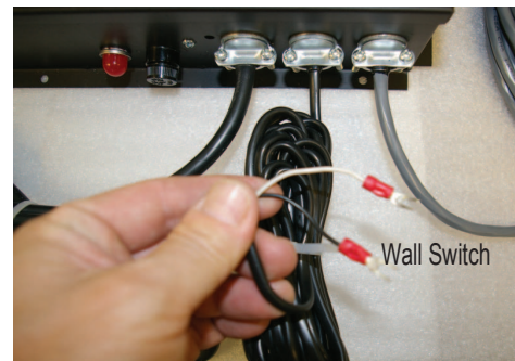
Figure 15c. (Remote Switch Wire connection)
